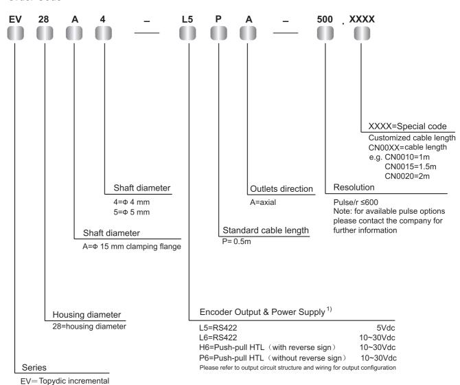
1)When UB=5V,short-circuit to channel, 0V,or+UB is permitted; When UB is greater than 5V, short-circuit to channel or 0V is permitted
